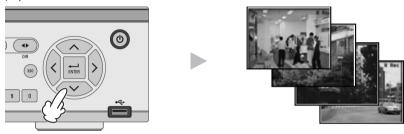
Press the ENTER button, and the four connected channels are displayed in quad split screen
